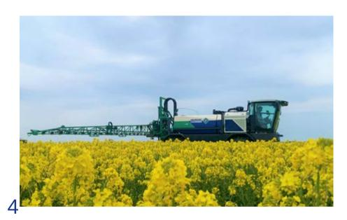
The Harrier is built on an advanced, single piece chassis complete with supremely robust A-Frame axles both front and rear. Power comes from an MTU 6R1000 6 cylinder Stage V engine providing 240hp, which is fully compliant with current emission legislation.
