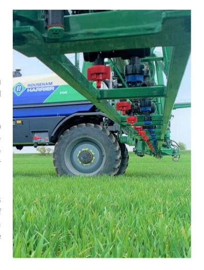
**HOUSEHAM BOOM LEVELLING** Designed to maintain a constant nozzle height over the crop canopy, boom levelling technology optimises spray dispersion and efficiency while minimising drift. As a result, operators can work faster and operate in more challenging conditions, reducing the impact of wind. The system uses sensors along the boom to monitor its position, multiple times a second, adjusting the boom height constantly.
