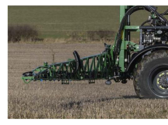
**HOUSEHAM BOOM LEVELLING** Designed to maintain a constant nozzle height over the crop canopy, boom levelling technology optimises spray dispersion and efficiency while minimising drift. As a result, operators can work faster and operate in more challenging conditions, reducing the impact of wind. The system uses sensors along the boom to monitor its position multiple times a second, adjusting the boom height constantly.
