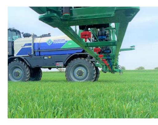
**HOUSEHAM BOOM LEVELLING** Designed to maintain a constant nozzle height over the crop canopy, boom levelling technology optimises spray dispersion and efficiency while minimising drift. As a result, operators can work faster and operate in more challenging conditions, reducing the impact of wind. The system uses sensors along the boom to monitor its position multiple times a second, adjusting the boom height constantly.
