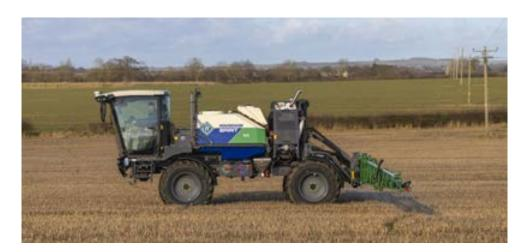
The Spirit is built on an advanced, single piece chassis complete with enhanced A-Frame axles both front and rear. Power comes from an MTU 4R1000 4 cylinder Stage V engine providing 170hp.
