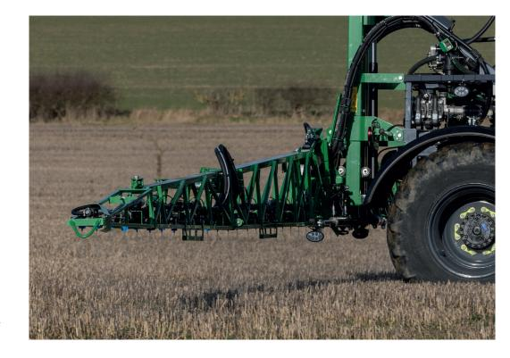
**HOUSEHAM BOOM LEVELLING** Designed to maintain a constant nozzle height over the crop canopy, boom levelling technology optimises spray dispersion and efficiency while minimising drift. As a result, operators can work faster and operate in more challenging conditions, reducing the impact of wind. The system uses sensors along the boom to monitor its position multiple times a second, adjusting the boom height constantly.
