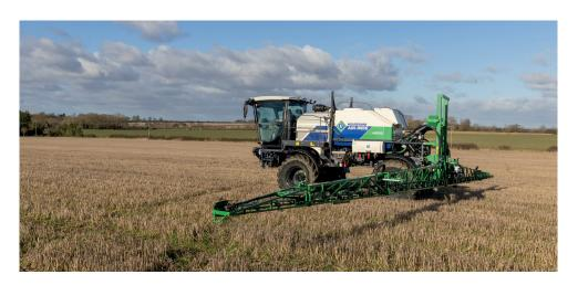
The Air-Ride is built on Househam's proven low-weight chassis that features active load-sensing air suspension for a class-leading ride whatever the terrain. Power comes from an MTU 4R1000 4 cylinder Stage V engine proving 170hp.
