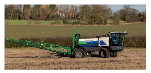
The Harrier is built on an advanced, single-piece chassis complete with supremely robust A-Frame axles both front and rear. Power comes from an MTU 6R1000 6-cylinder Stage V engine providing 240hp, which is fully compliant with current emission legislation.
